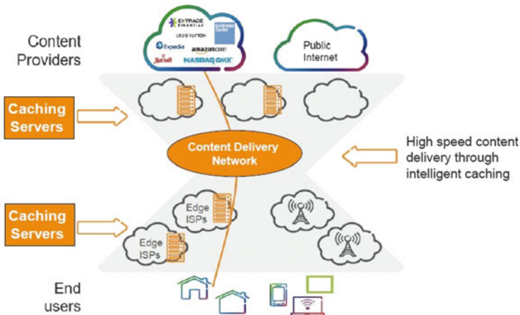
Fig. 7.8 Efficient Internet content delivery architecture through CDN and caching servers
